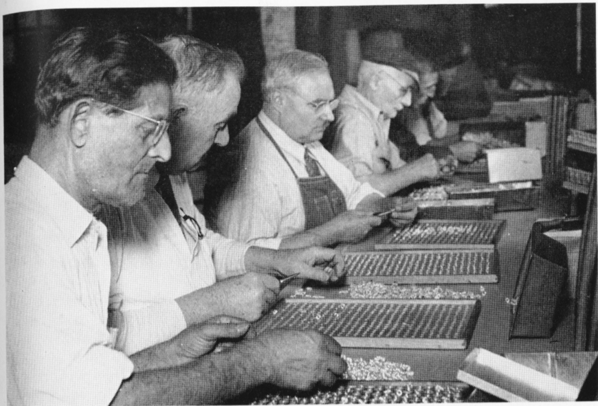
The Repair Room, operating under Freddie Ayotte, saves time, money and materials for the Company and today for the war effort. Here Ignazio Buscema, Francis Kirley, Constantino Calvo, George Gentil, Ed Kleps and Egbert Holden disentangle Camloc springs recently shipped to Scovill.
