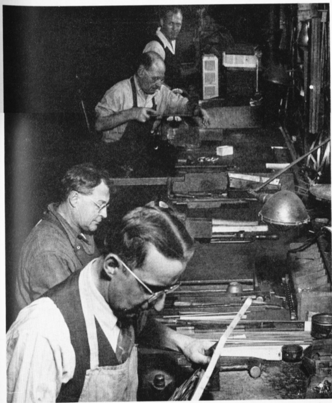
This is the rack-makers' bench. A few racks are made in the Plating Room, but the majority are made here by men who have been at the job for years. The Repair Room renders some service to every department in the Plant. They do several light manufacturing jobs on foot and power presses. The room's greatest distinction is perhaps the fact that it is the only mechanical department in existence today that has run since it was born without as much as one lost-time accident. For a room working with the machinery which these men operate, this is a record to which they may truly point with pride.
